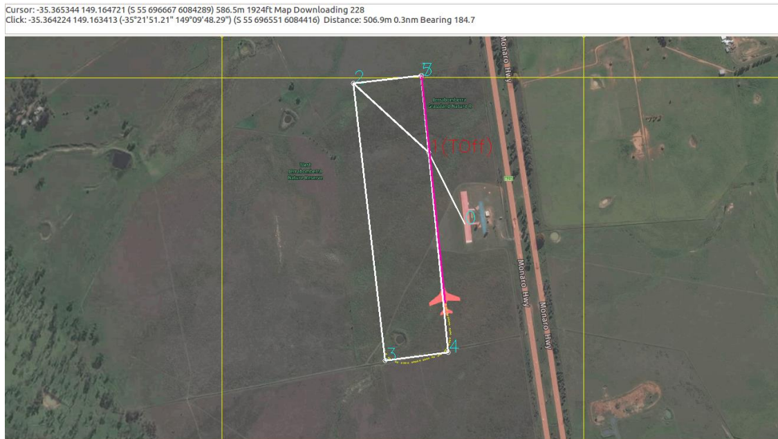
Figure 7.2 Map of the waypoints loaded for UAV navigation in SITL environment.
