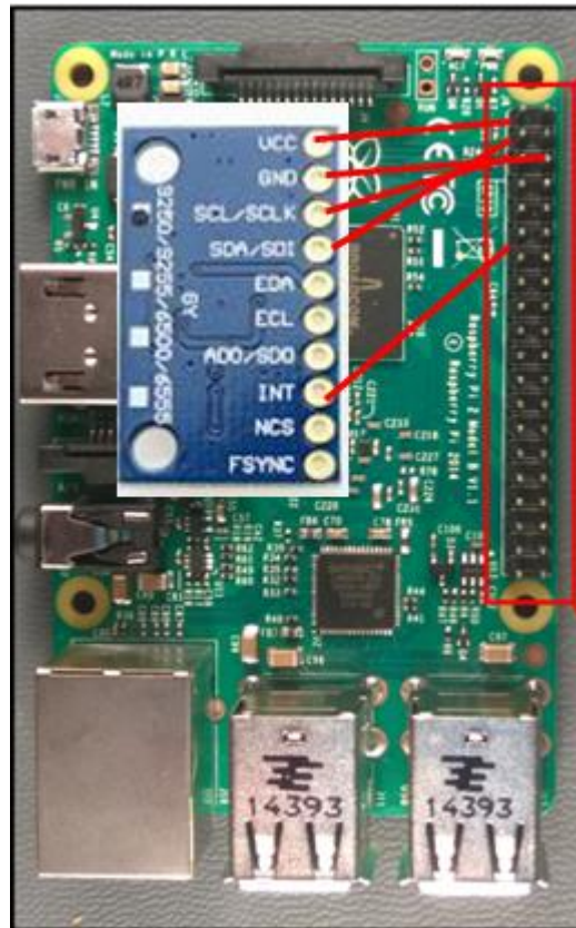
Figure 8.3 Connection pins of the MPU-9250 and GPIO pins of Raspberry pi.
